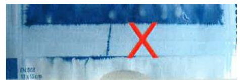
Fig. 3: Negative test. Test solution penetrates the sealing seam.
