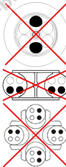
Fig. 6: Permissible and impermissible loading of an angle rotor and a swing-out rotor (example illustrations)
