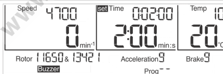
Fig. 12: Setting the runtime, here in the time unit "min:s"
