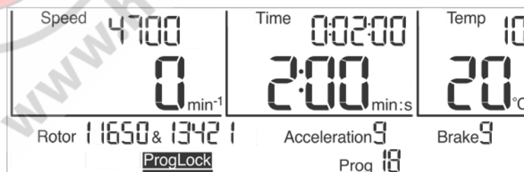
Fig. 22: The program lock "ProgLock" is activated
