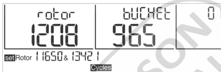
Fig. 23: Cycle display for rotor 11650 and bucket 13421
