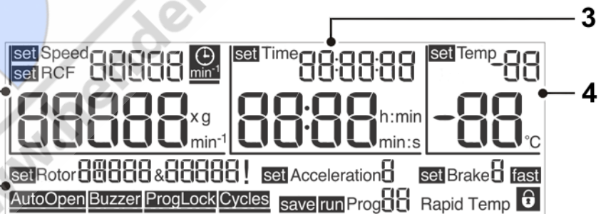
Fig. 10: Display of the Spincontrol L control system
