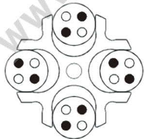
Fig. 8: Permissible and impermissible loading of an angle rotor and a swing-out rotor (example illustrations)
