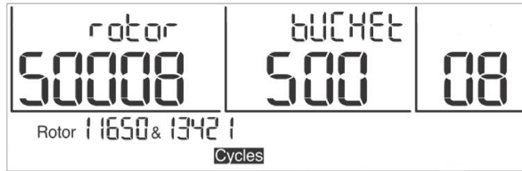
Fig. 23: Display when the maximum number of cycles is reached (flashing)
