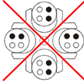
Fig. 8: Permissible and impermissible loading of an angle rotor and a swing-out rotor (example illustrations)
