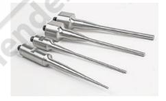
**Micro Tips:** These smaller, high-intensity tips are ideal for processing smaller samples in Eppendorf vials or similar vessels. Available in stepped or tapered designs. Sizes range from 3/32" to 1/4".
